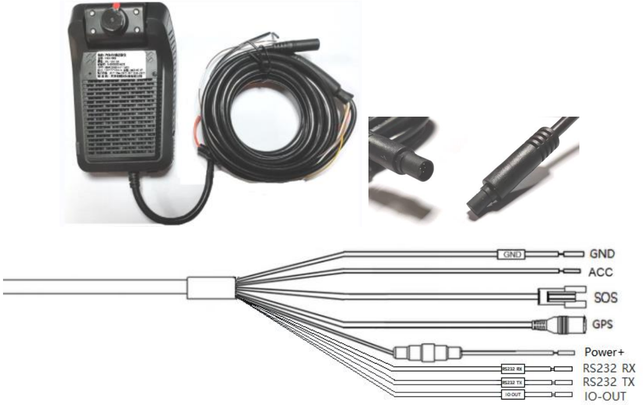
Picture 2. Power line interface definition
