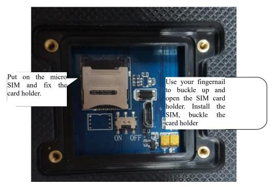
2. Turn the switch to the ON position to turn on the smart lock.
