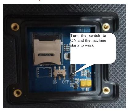
3. Install the SIM and turn on the battery switch, close the bottom cover, and attach the screw
