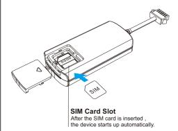
NOTE A SIM card is required for SMS, data services and calling functions(Calling needs phone card).
