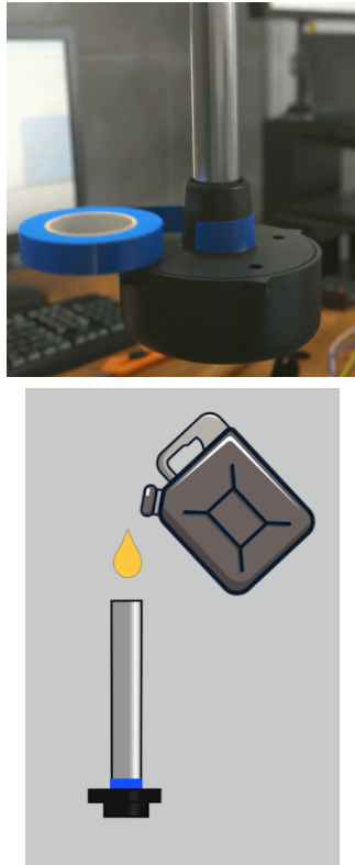
Fig. 17 Covering drainage hole, turning the sensor upside down and filling the tubes from a jerry can
