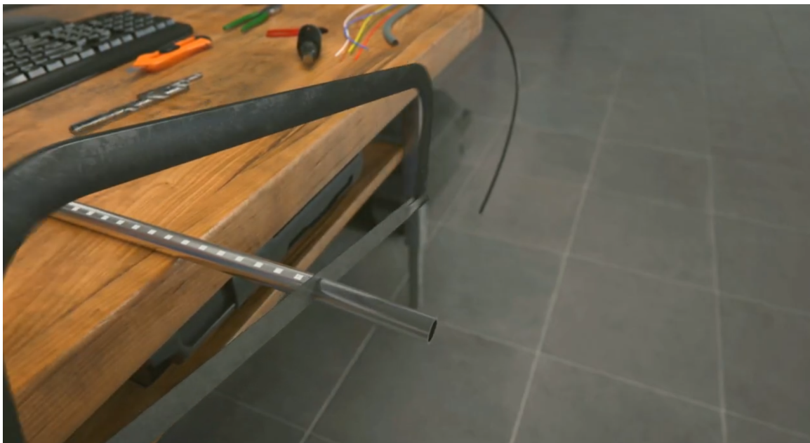
Fig. 37 Cutting the tubes
