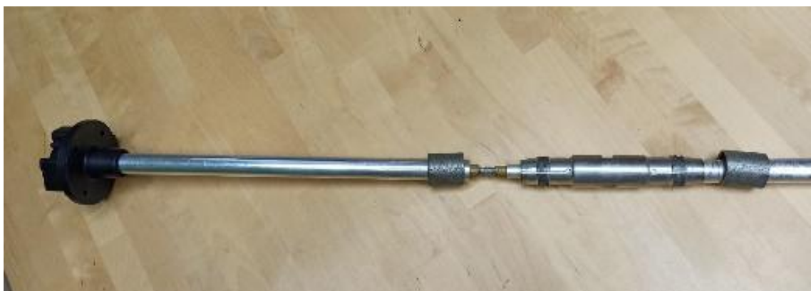
Fig. 39 Collet coupling. Inner coupling
