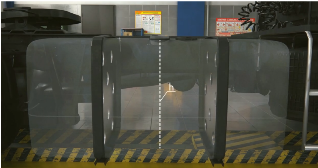
Fig. 35 Measuring the height of the tank
