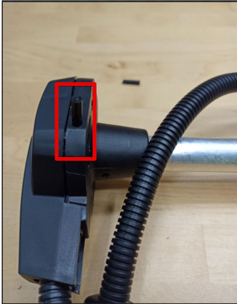
Fig. 87 Push the dowel into the orifice
