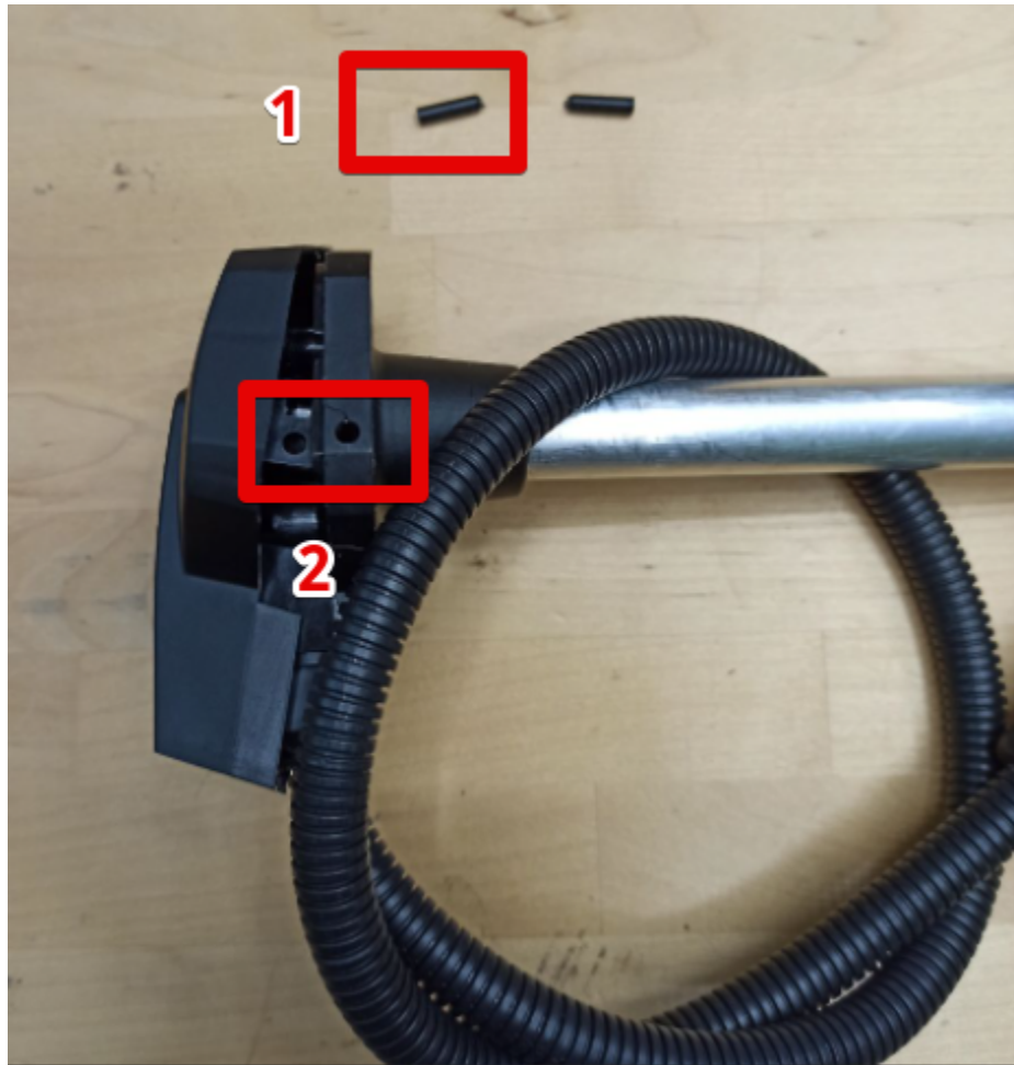
Fig. 86 Putting the protection case and aligning sealing orifices
