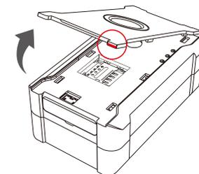
Find the notch and open the device casing
